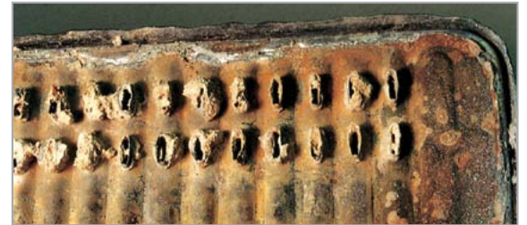
Neglected Cooling System
