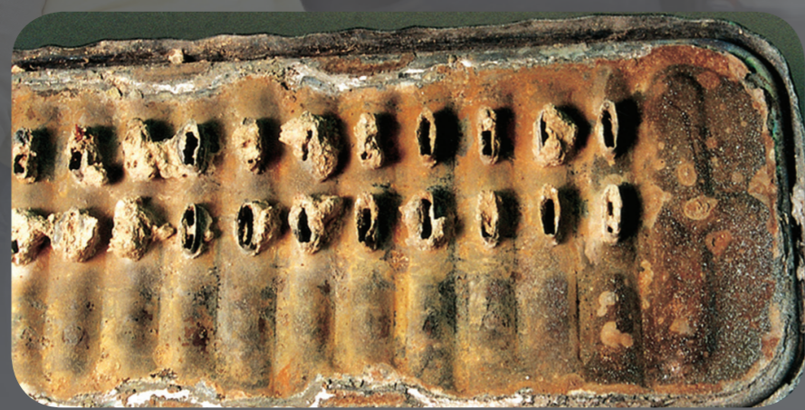
Dirty Neglected Radiator
