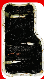
Dirty neglected Engine Oil System.
